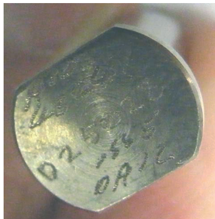
Above: The hinge pin which was removed from Servo Commande assembly, which shows the Meggitt identification markings on it.
