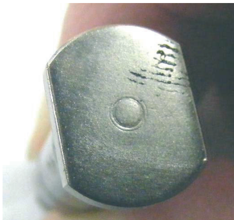
Above: The hinge pin which was removed from Servo Commande assembly, which shows no identification markings on it.
