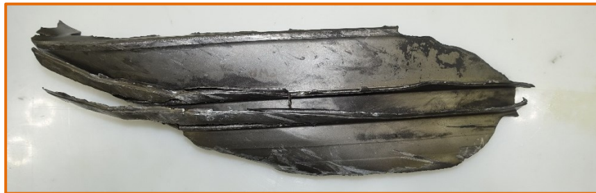
First stage of low pressure compressor of the engine
