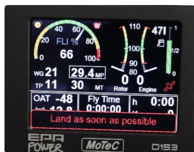
Figure 6: New display of engine parameters in the event of an error message
