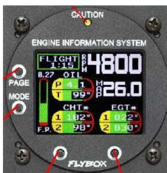
Figure 3: Example of display of essential engine parameters on the Mini EIS
