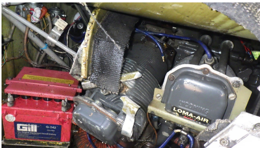
Figure 2: Right rear cylinder separated from crankcase
