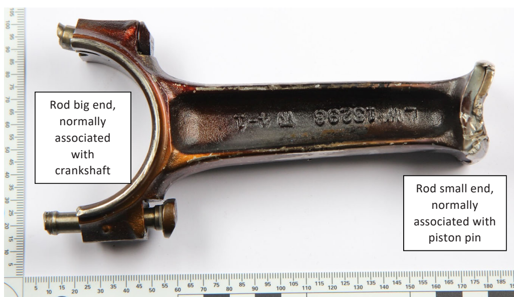
Figure 5: Rod of cylinder 3
