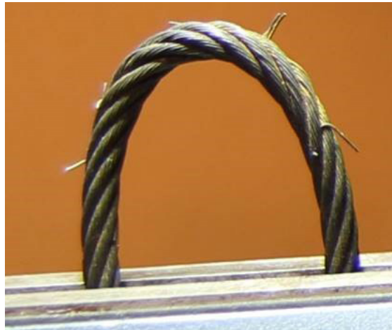
Figure 6: Position B of the RH cable with presence of broken wires upstream of pulleys, pedal in neutral (cable bent using a vice in the laboratory to provide a better view of the broken wires)
