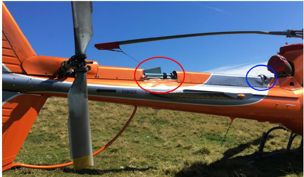
Figure 3: External damage on the tail boom
