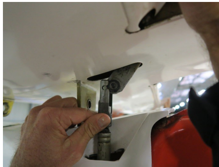
Figure 7: Positioning elevator lever bolt on quick-release end (sleeve in the down position)
