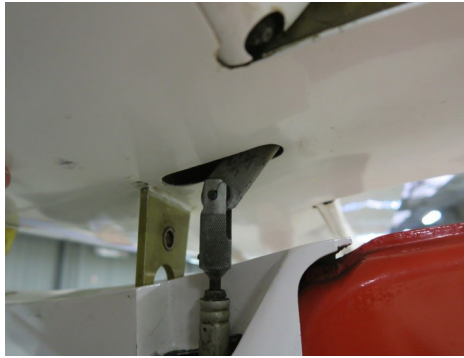
Figure 9: Connection made and sleeve locked with the spring system in its up position (secure connection)
