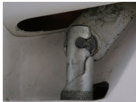
Figure 8: Connection made between elevator lever bolt and quick-release end (sleeve in the down position)
