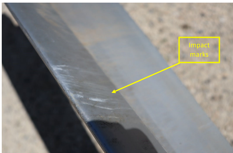
Figure 5: Marks observed on the main rotor blades
