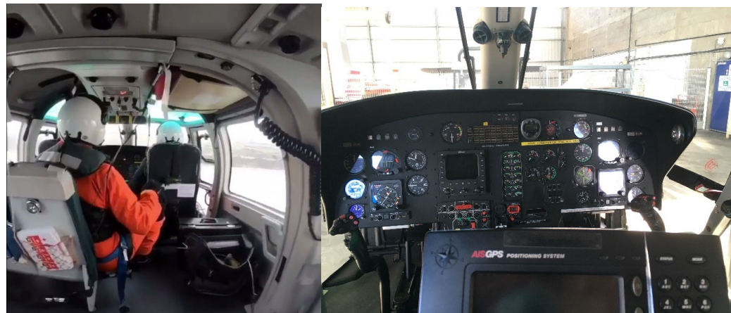
Figure 2: cabin configuration and view from the hoist operator's place
