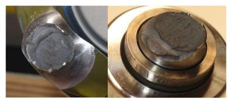
Figure 19: Trunnion pin fracture surface (on left, tulip side, on right, end of trunnion pin side)
