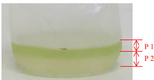
Fuel and water recovered from the left carburettor bowl
