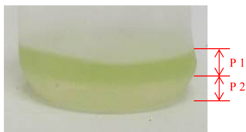
Fuel and water recovered from the right carburettor bowl
