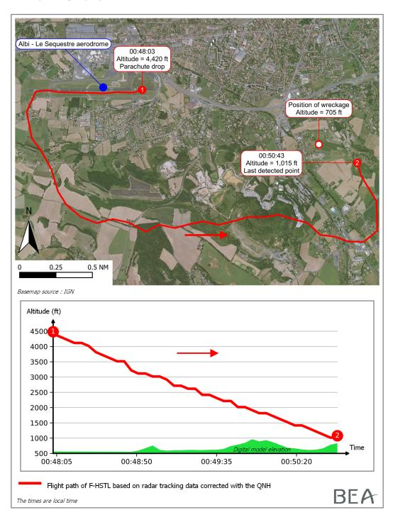
The examination of the flight path found that the average rate of vertical descent was constant during the last minute of the flight and was approximately 1,100 ft/min. The glide path did not show any dip that would be consistent with a loss of engine power. The glide path was constant up to the radar detection limit near the accident site. At that point, its height was approximately 200 ft.
