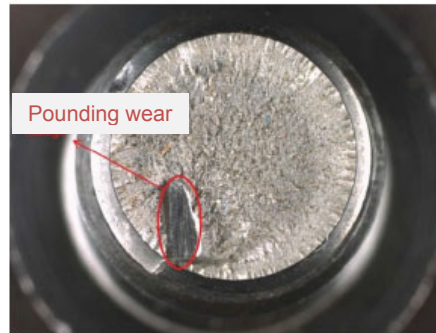
Figure 7: Photo of the fractured face (nut side)
